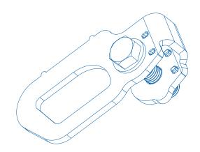
The Rapid Rail International SK-2 solves the problem of step bolts not meeting anchor point standards. The SK-2 is simply fitted to an existing step bolt which then becomes a 5000lb (22kN) rated anchor point and can be left in place once fitted for future use.
