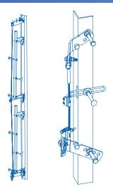
The Rapid Rail International Vertical Cable System (VCS) is a wire rope-based fall arrest system designed for installation to electrical transmission and distribution towers and poles, telecoms towers and other similar structures. The VCS2 system offers permanent attachment and fall arrest protection for up to four climbers working simultaneously and arrests falls within 2ft.
